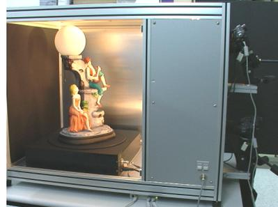
Figure 8. An experimental setup consists of two static color cameras and a turntable on which concentric circle patterns are printed for calibration.
