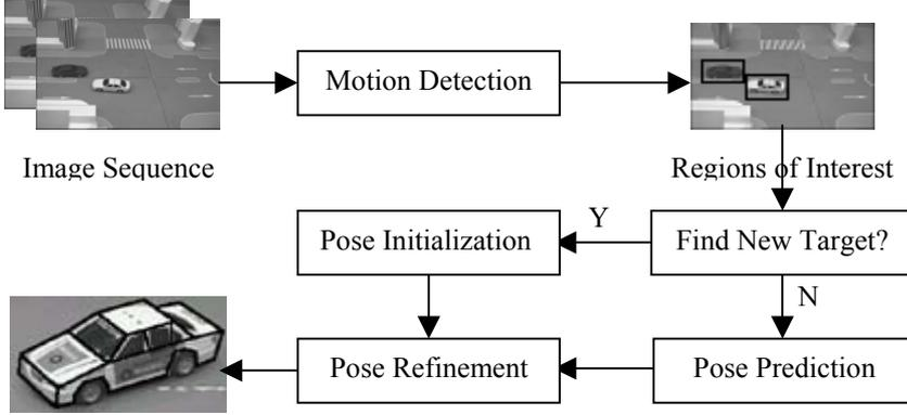
Figure 1. Overview of our tracking system (The camera is static and calibrated, and 3D wireframe models are used.)
