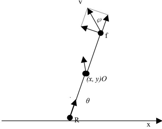
Figure 2. The bicycle model of car motion
