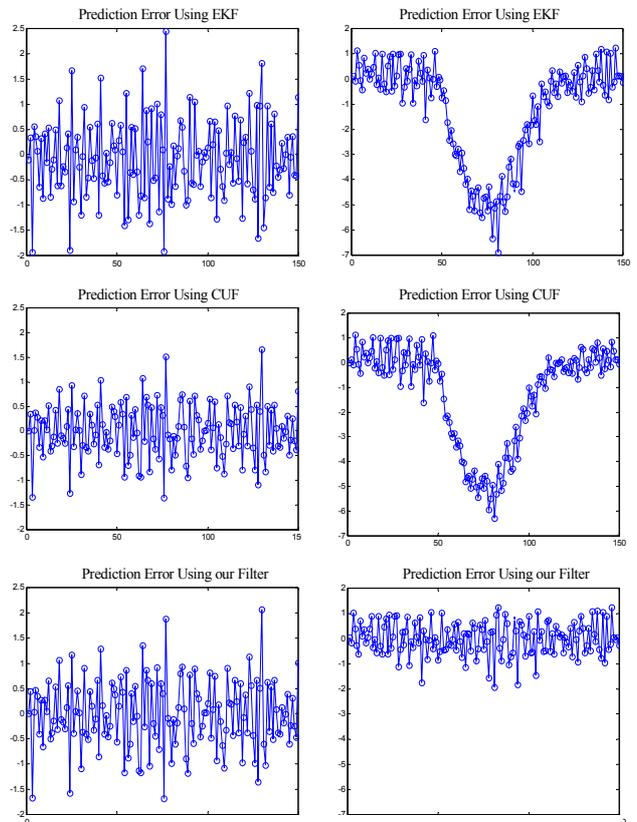
Figure 5. Prediction errors (between prediction and ground truth) of an EKF predictor,
