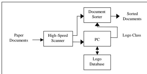
**Figure 1. Example application where logo recognition facilitates the automatic sorting of paper documents according to corporate identity**
