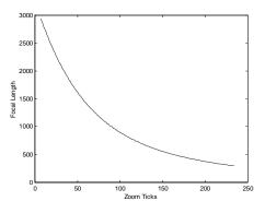
**Figure 2**: Typical curve showing focal length as a function of zoom ticks.
