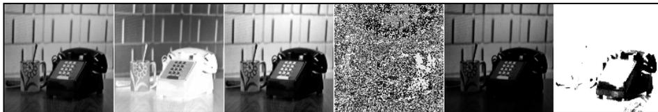
Fig. 2. Processed Image for *Phone* Image (From left to right): original image, image inversion, random intensity mapping, image equalization, squared intensity mapping with normalization, and squared intensity mapping with clipping.
