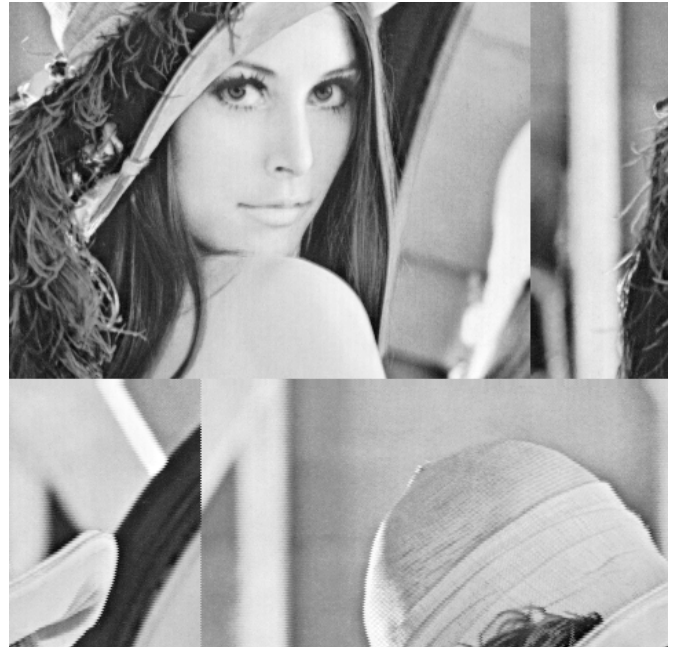
Figure 1. Reconstructed image after translation by offsets dx = 100 and dy = 200 in R(t, m) space (479 x 479 image).
