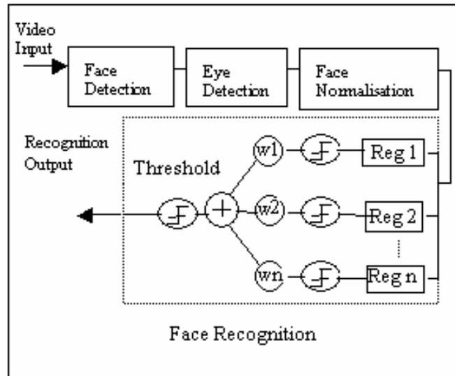
Figure 2: Block Diagram of a Multi-region Feature Face Recognition System
