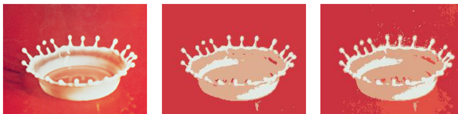
(a) (b) (c) Figure 4. (a) the original image “Splash”; (b) the final results with three colors obtained by the proposed method with h=7 ; (c) the results with six colors without considering the local homogeneity and the cyclic property of the hue ( h=7 ).
