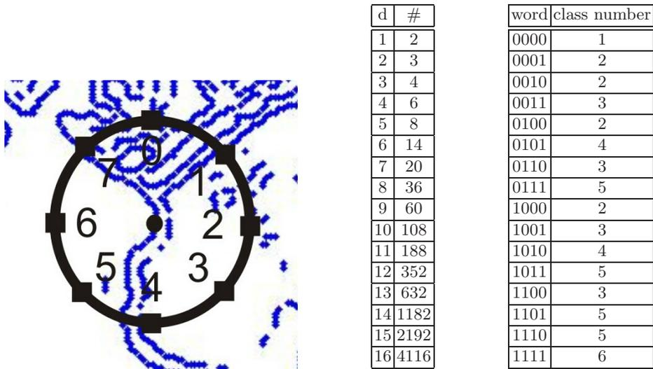
**Fig. 2.** Left: a binary string of pixels centred at each edge point is mapped to an invariant class. Middle: number of equivalence classes (#) in relation to the length of the binary string ( $d$ ). Right: an example of a function table for  $d = 4$ .
