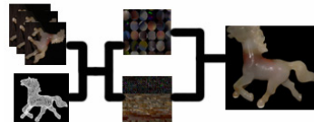
Fig. 1. The pipeline of edge-based non-uniform LFM. Left: acquired images and geometry of the object. Middle: view textures and surface textures. Right: rendering result
