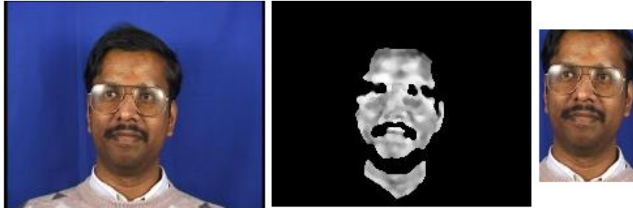
Fig. 3. Grouping example. Although the neck is separated from the face, the two components are still treated as a single group. From left to right: Original image; Median image that resulted from \lambda_{i,j}^2 calculations; minimal rectangular region that contained the pixels labeled as skin.
