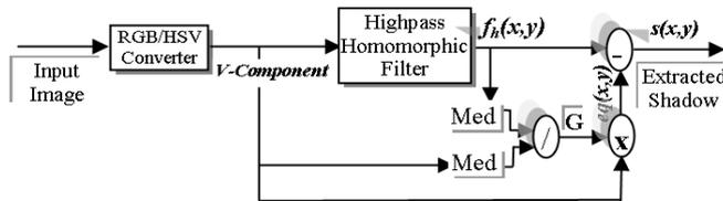
Fig. 5. Block diagram of the proposed system using HPP
