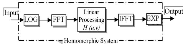
Fig. 2. Block diagram of the homomorphic system
