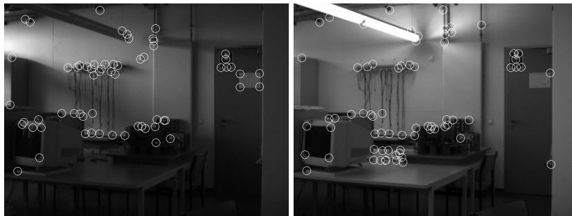
Fig. 1. In the left image the scene is illuminated by sunlight, whereas in the right image the light comes from neon lamps. The detected interest points are indicated by circles of radius 3\sigma . Here T = 0.01 \cdot \max(R) is used as proposed in [10]. Only 46.0% of the interest points of the left image are re-detected in the right image.
