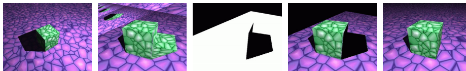
Fig. 2. The first pass computes the depth to each point visible by the source camera ( i ). The second pass textures the scene ( ii ). The third pass tests the depth of each fragment with the shadow map ( iii ).
