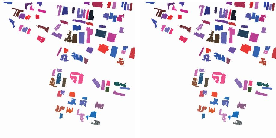
**Fig. 6.** Buildings extracted in the first (left) and third (right) iterations.
