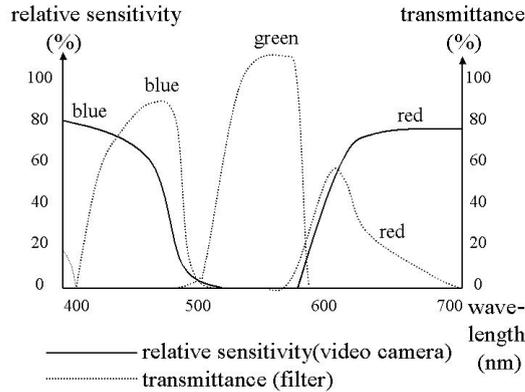
**Fig. 2.** Relative sensitivity of the video camera and transmittance of the red and blue filters.
