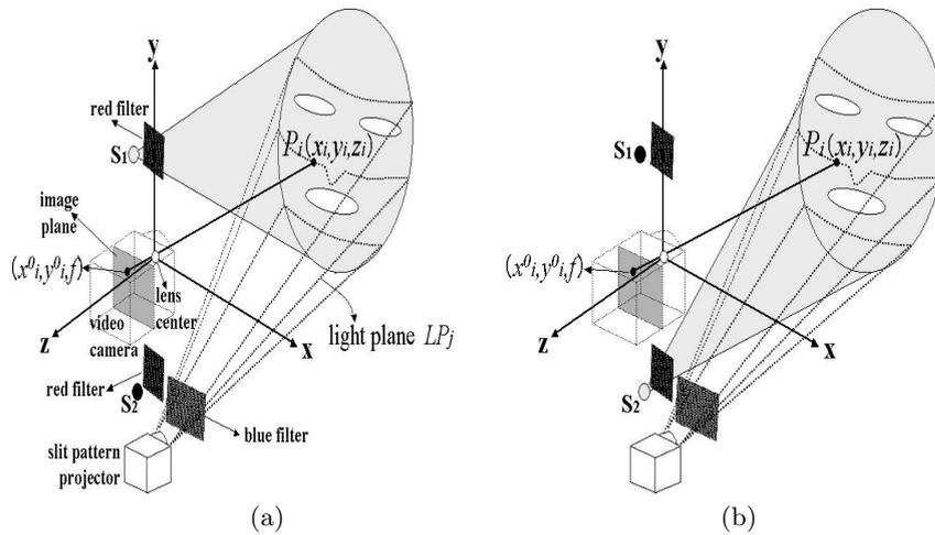
**Fig. 1.** Two point light sources  $S_1$  and  $S_2$  are switched in turn to illuminate the face, while a slit pattern projector illuminates the face all the time. (a) The face is illuminated by  $S_1$  and the slit pattern projector. (b) The face is illuminated by  $S_2$  and the slit pattern projector.
