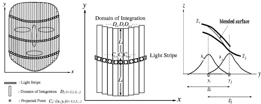
**Fig. 3.** Division of the surface region. **Fig. 4.** The domain of integration. **Fig. 5.** Surface blending procedure.
