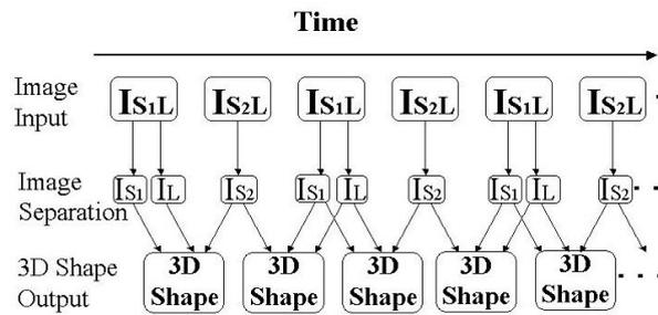
Fig. 10. Time sequence of the measurement process.
