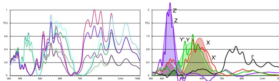
**Figure 6** 6-channel triple diode color sensor: measured spectral response and corrected functions with CIE XYZ for comparison
