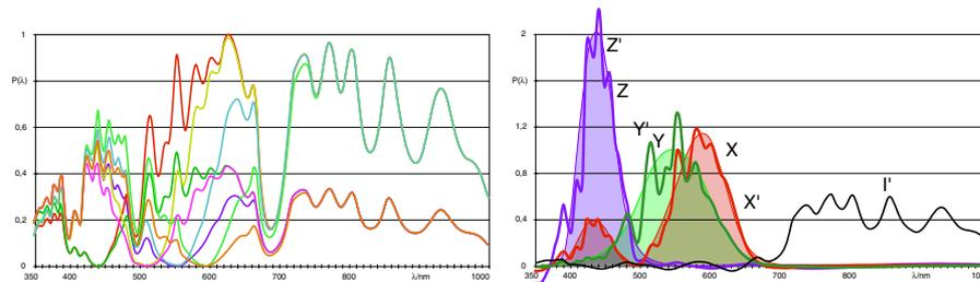
**Figure 7** 8-channel dual diode color sensor: measured spectral response and corrected functions with CIE XYZ for comparison
