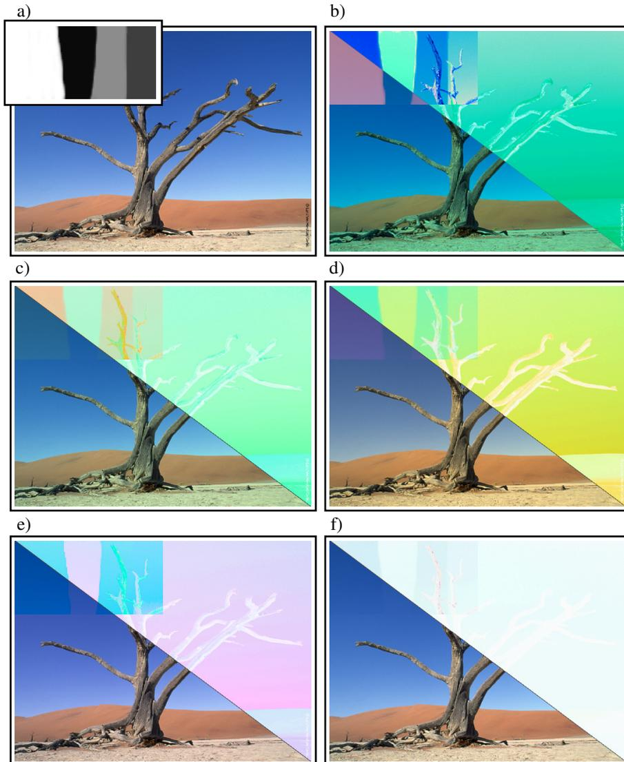
**Figure 9** Simulation Results: a) Reference image with an additional infrared distortion; b) 3-channel Bayer mosaic sensor; c) 4-channel color correction (Figure 4); d) 4-channel dual diode; e) 6-channel triple-diode (Figure 6); and f) 8-channel dual diode sensor (Figure 7).
