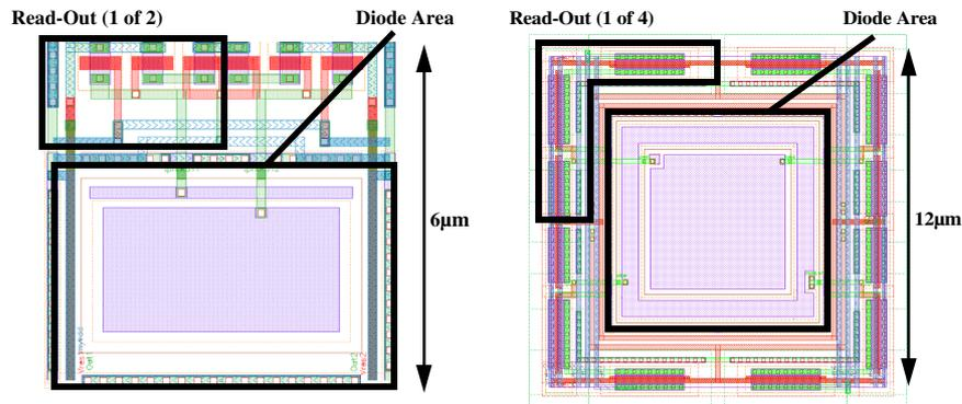
**Figure 10** a) Dual Junction Photo Diode and b) Triple/Quad Junction Photo Diode; layout sample with circuitry for read-out
