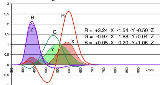
**Figure 1** Theoretical sRGB spectral sensitivity with CIE XYZ
