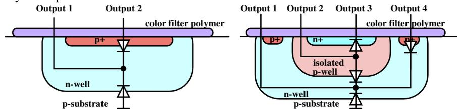
**Figure 5** a) Dual Junction Photo Diode and b) Triple/Quad Junction Photo Diode
