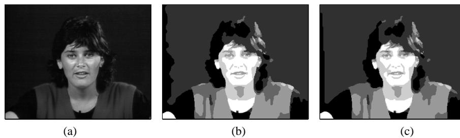
**Fig. 7.** Miss America image segmentation with  $k = 5$  clusters and  $\beta = 50$ ; (a) Miss America image  $288 \times 352$ ; (b) scalable segmentation; (c) scalable segmentation with smoothing constraint.
