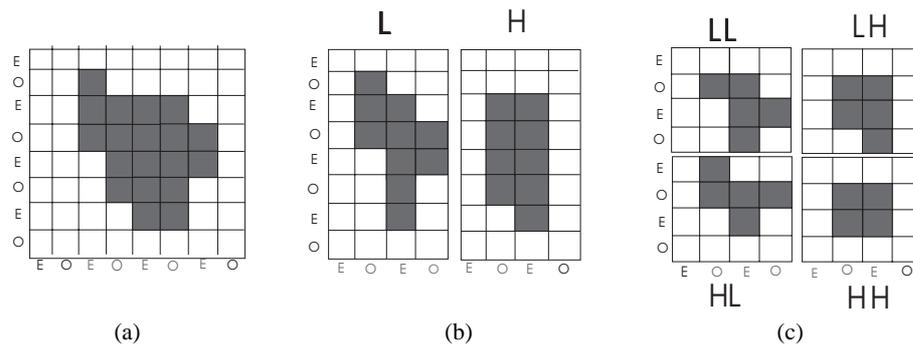
**Fig. 1.** Decomposition of a non rectangular object with odd-length filters; (a) the object, shown in dark gray; (b) the decomposed object after horizontal filtering; (c) decomposed object after vertical filtering. The letters "E" and "O" indicate the position(even or odd) of a pixel in the horizontal and vertical dimensions.
