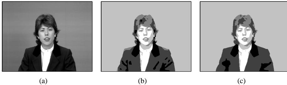
**Fig. 3.** Claire image segmentation with  $k = 5$  clusters and  $\beta = 50$ ; (a) the main image; (b) segmentation by the proposed algorithm; (c) regular multiresolution segmentation;
