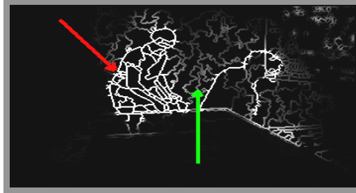
Figure 2: Illustration of RAG edges of one frame taken from the "Tennis" video sequence, after assigning gcp_i^{e(u,v)} weight for all e(u,v) \in E where i=5 comparisons.
