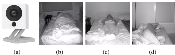
Fig. 15: Posture change validation. Camera used in the validation and images taken during the experiment. (a) The infrared camera with motion detection. (b) Lady sleeping on the right. (c) Second lady sleeping on the back. (d) Man sleeping on the left.
