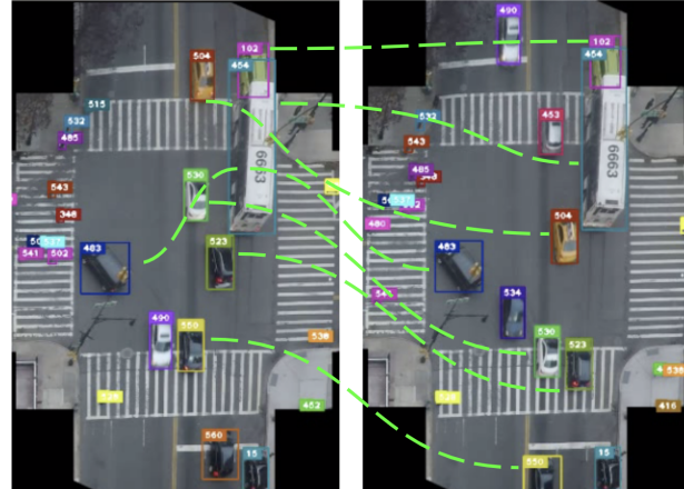
Fig. 5. Example of tracking output: Deepsort + MaskRCNN on frame 800 (right) and 825 (left)
