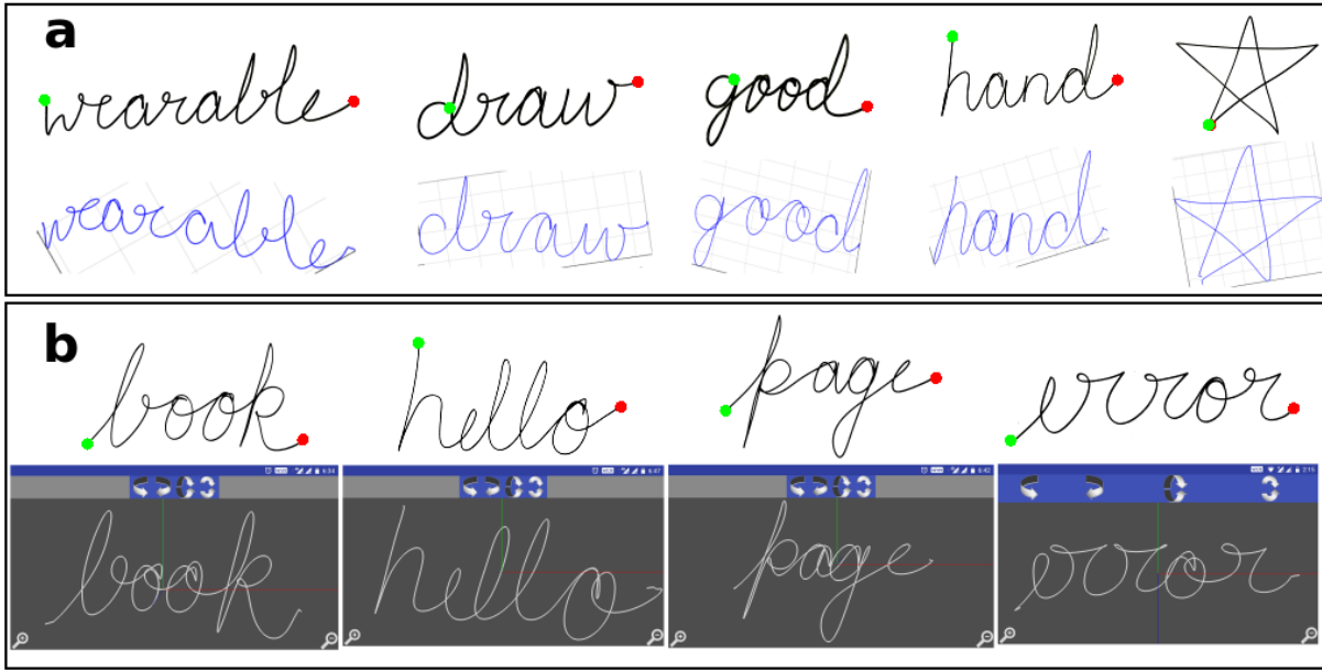
Fig. 4. Words digitally reproduced by AiRite, along with ground truth above each reproduction. (a) LG Urbane Smartwatch, and (b) Oneplus 5 Smartphone. Starting and ending points of tracing for a word are marked by green and red dot respectively.
