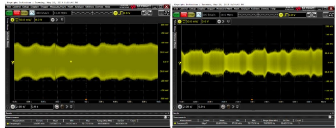
Fig. 10. Coupled voltage in the NFC receiving antenna, showing the modulated signals caused by the human respiration activities. (Left: normal breathing; Right: deep breathing.)
