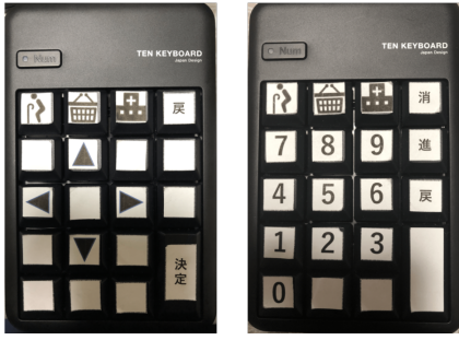
Fig. 5. Key Design (Left: Cursor Type, Right: Numeric Type)
