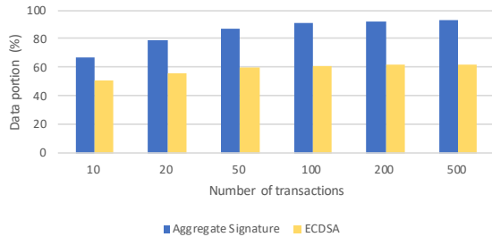
Fig. 5. Sensor data proportion in a block with or without aggregate signature.
