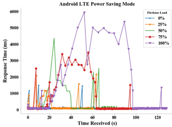
Fig. 6. Response time plot for Android LTE Power Saving mode
