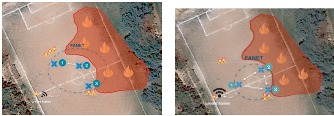
Fig. 4. Multi-hop scenario when the formed triangle is wider (left), where UAVs have multi-hop techniques to communicate, and non-multi-hop scenario (right) where UAVs are directly connected.
