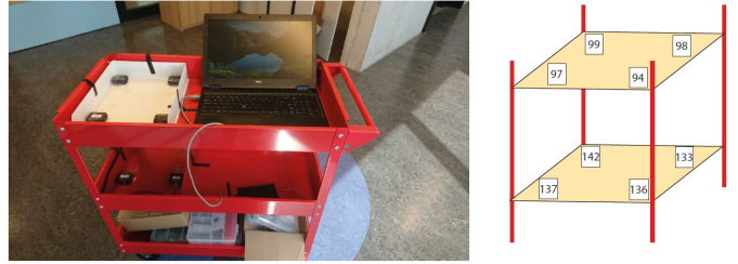
Figure 1. The experimental setup which mimics smart pallet is used to collect motion dataset.
