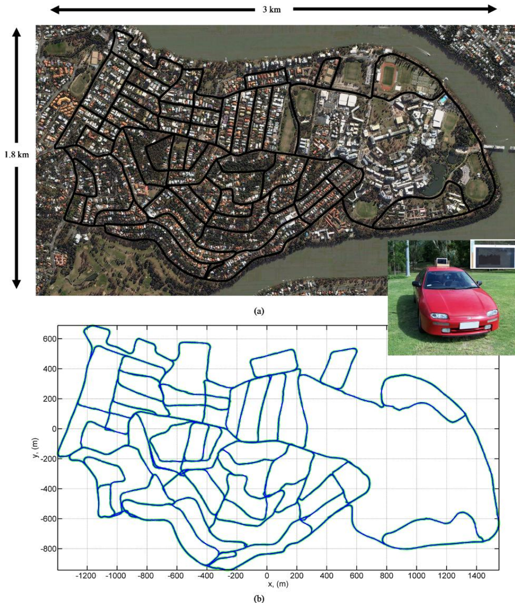
Figure 3. RatSLAM created an accurate street map of the entire suburb of St Lucia (66 km of driving) using only the sensory input from a web camera mounted on top of the car.
