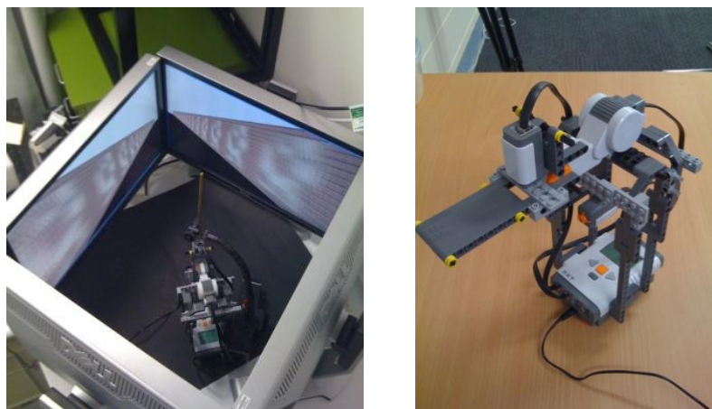
Figure 8. (left) Four monitors with moving scene surrounding the Bee tether and LEGO platform. (right) The LEGO platform from another angle.
