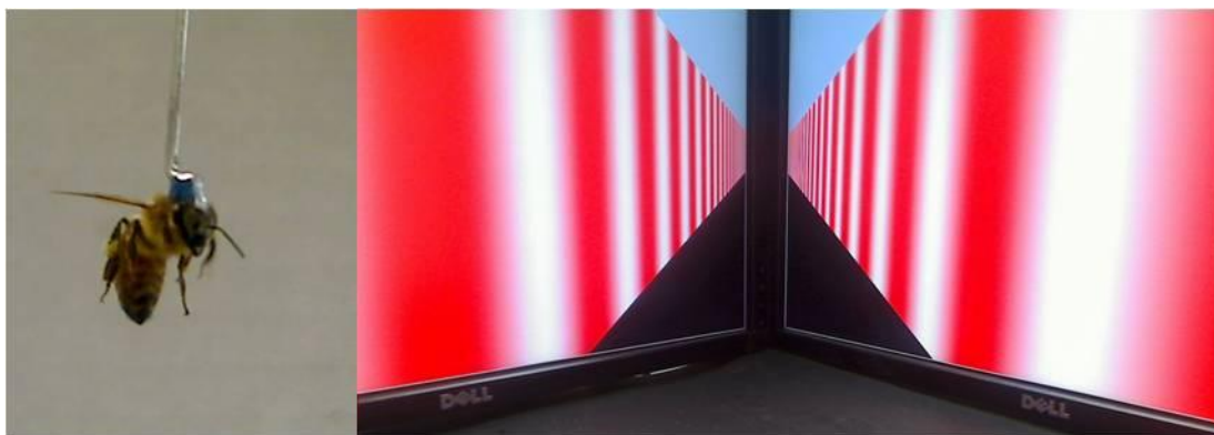
Figure 1: (a) Tethered honeybee, (b) View of tethered bee in virtual-reality arena.
