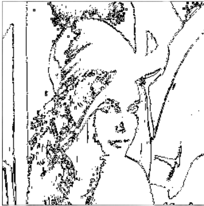
Figure 6. 256x256x8-bit Lena: Output of NN edge detector trained to duplicate "fuzzy" Sobel edgedness on 256 binary proto-types. Number of edge pixels = 7770.
