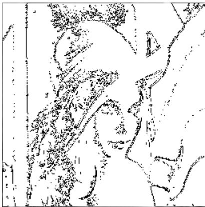
Figure 7. 256x256x8-bit Lena: output of nn edge detector trained to duplicate "de-fuzzified" sobel edgedness on 256 binary proto-types. Number of edge pixels = 5895
