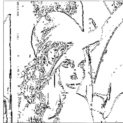
Figure 8. 256x256x8-bit Lena: Output of NN edge detector trained to duplicate Sobel edgedness on 40 "crisp" proto-types. Number of edge pixels = 6852
