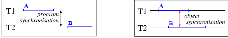
Fig. 7. Scenarios of synchronisations between threads
